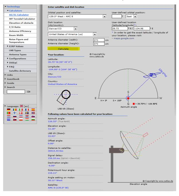
6. Drop down the orbital position and satellite box in step 2 to select "105.0West: AMC15/18", select "calculate" and make note of the new data.
